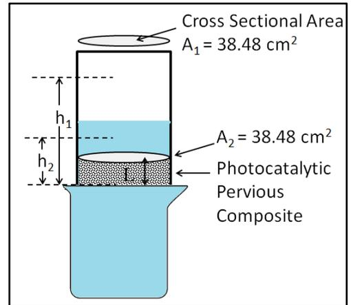
**Figure 5.** Schematics of the falling head test
