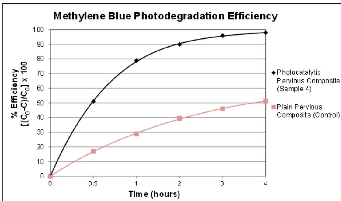
**Figure 8.** Methylene blue photodegradation efficiency for the photocatalytic pervious composite and the plain pervious composite
