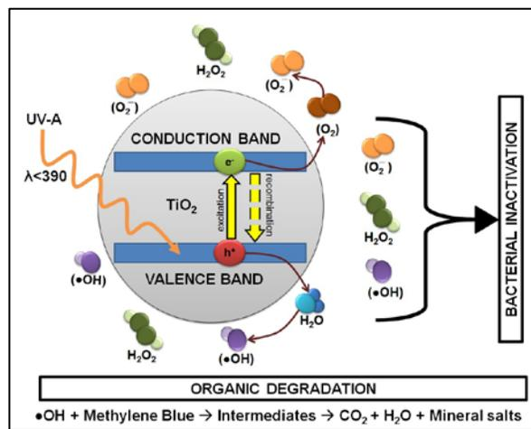
**Figure 1.** Bacterial inactivation and organic degradation by advanced oxidation process
