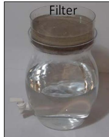
**Figure 11.** POU photocatalytic filter
